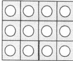
**FIGURE 3.** Periodic structure of a composite material
