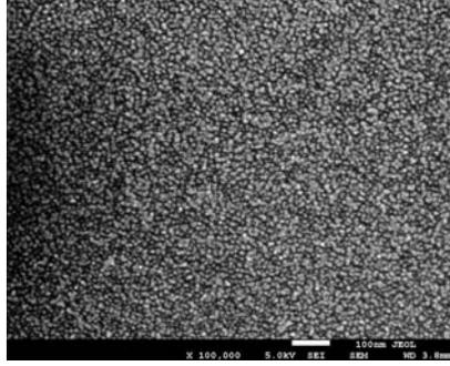
**FIGURE 2.** TEM image of a fragment of real Pd-carbonaceous nanocomposite material
