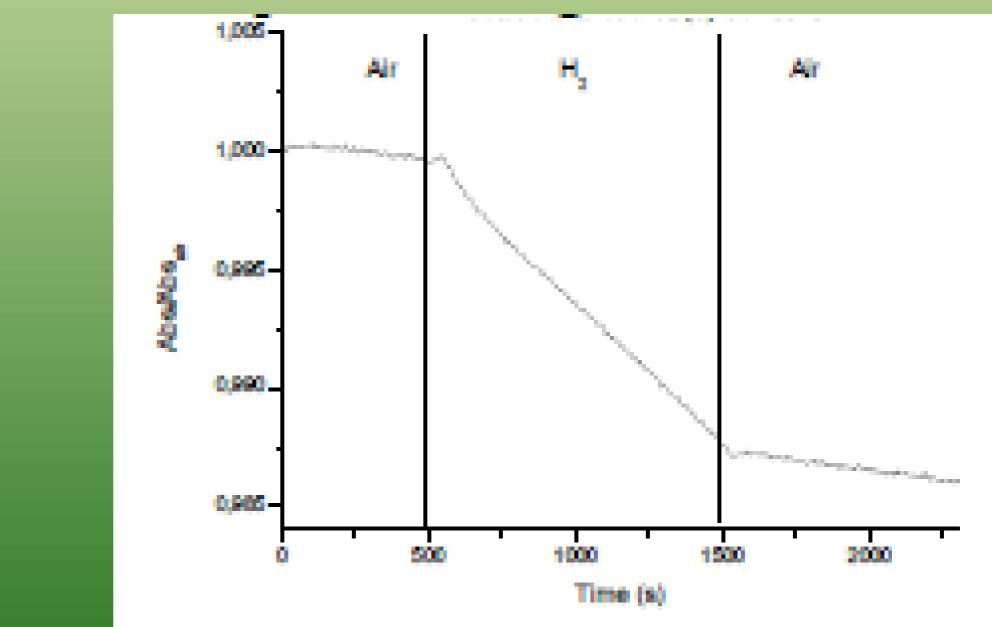
Dynamic scan of the sample B2 at OT=80°C and  $\lambda$ =1050nm
