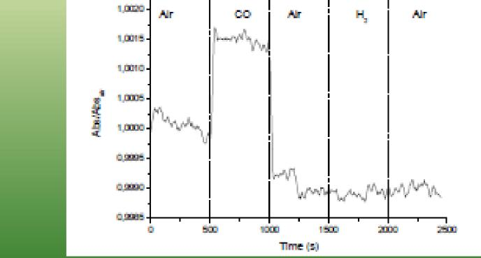
Dynamic scan of the sample S1 at operating temperature  $OT=80^{\circ}C$ ,  $\Lambda=2325$ nm
