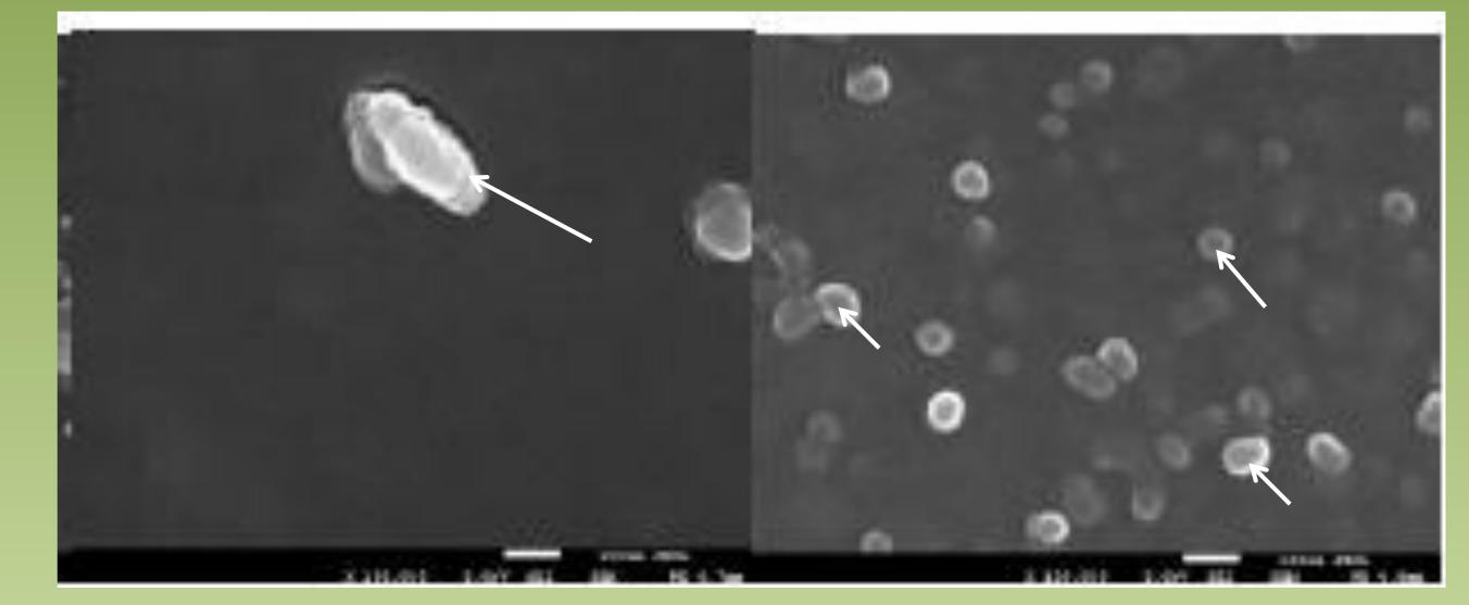
Sample A2 sample B2 Pd nanograins covering nanotubes are marked with white arrows
