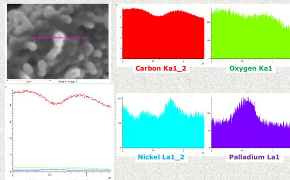
Our films possesses low resistance of order 100 Ohm, what could be connected to a Pd nanograins palced all over each nanotube
