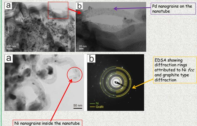
Our films were prepared by mixed PVD/CVD/PVD methods. Firstly nanocomposite film built of Ni and carbonaceous nanograins was deposited on a substrate by PVD method. Then, in CVD pyrolytic method a film of multiwall carbon nanotubes were obtained. Finally, nanograins of Pd and fullerenes were deposited on such film also by PVD.
