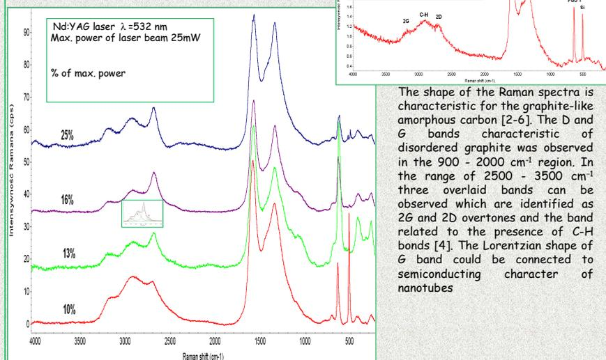
The shape of the Raman spectra is characteristic for the graphite-like amorphous carbon [2-6]. The D and G bands characteristic of disordered graphite was observed in the 900 - 2000  $\text{cm}^{-1}$  region. In the range of 2500 - 3500  $\text{cm}^{-1}$  three overlaid bands can be observed which are identified as 2G and 2D overtones and the band related to the presence of C-H bonds [4]. The Lorentzian shape of G band could be connected to semiconducting character of nanotubes
