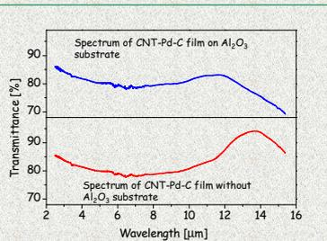
The top spectrum refers to CNT-Pd-C film deposited on alundum substrate and the bottom spectrum to CNT-Pd-C film after alundum substrate background subtracting. The presented spectra show that the films are transparent in far infrared region. The films transmittance decreases at the end of the spectral range. These films require further study in the MIR region.
