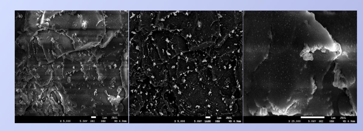
SEM images of the film C2 from a) SE detector, b) LABE detector and c) SE detector (a and b with x 5 000 magnification, c with x 25 000 magnification)
