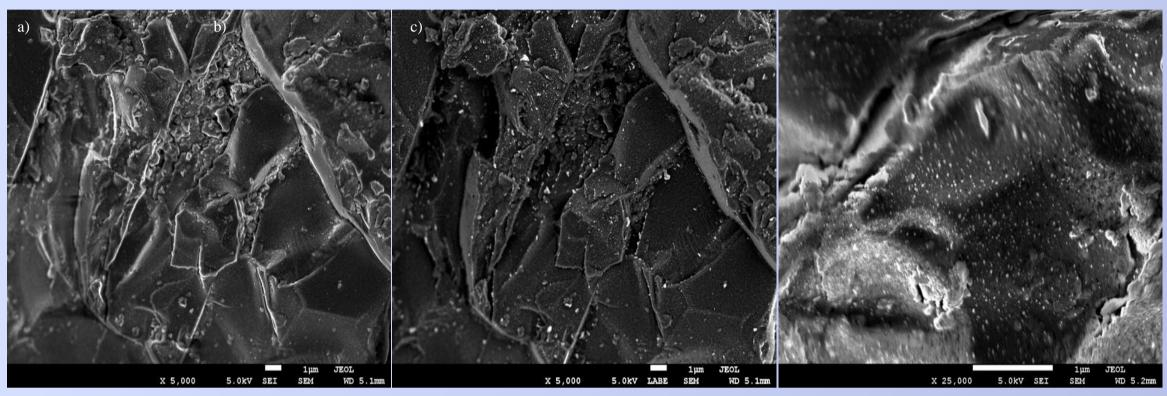
SEM images of the film C1 from a) SE detector, b) LABE detector and c) SE detector (a and b with x 5 000 magnification, c with x 25 000 magnification)
