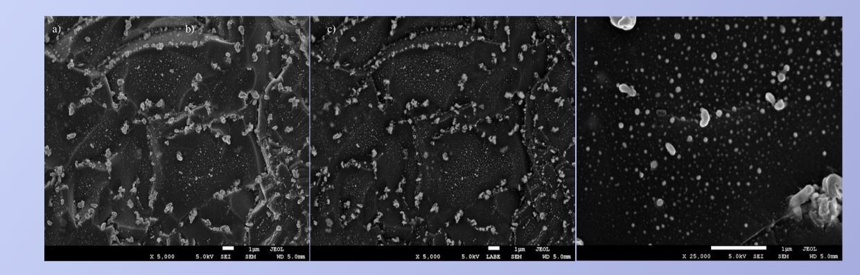
SEM images of the film C3 from a) SE detector, b) LABE detector and c) SE detector (a and b with x 5000 magnification, c with x 25 000 magnification).
