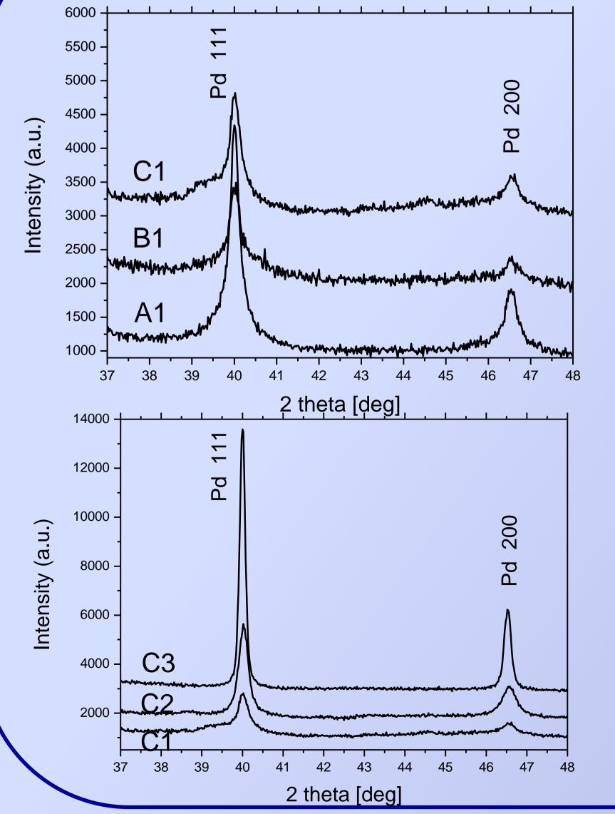
GIXD diffraction patterns of films A1, B1 and C1 (from annealing process at 500 °C)
